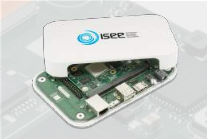
The expansion board is a fully equipped baseboard that access to almost all IGEP™ SMARC™ iMX6 functionalities. It has been designed to be used as the fastest way to develop and check the user's final application before building a prototype, saving costs and reducing time to market. This model can be used with all the IGEP™ SMARC™ series modules.
