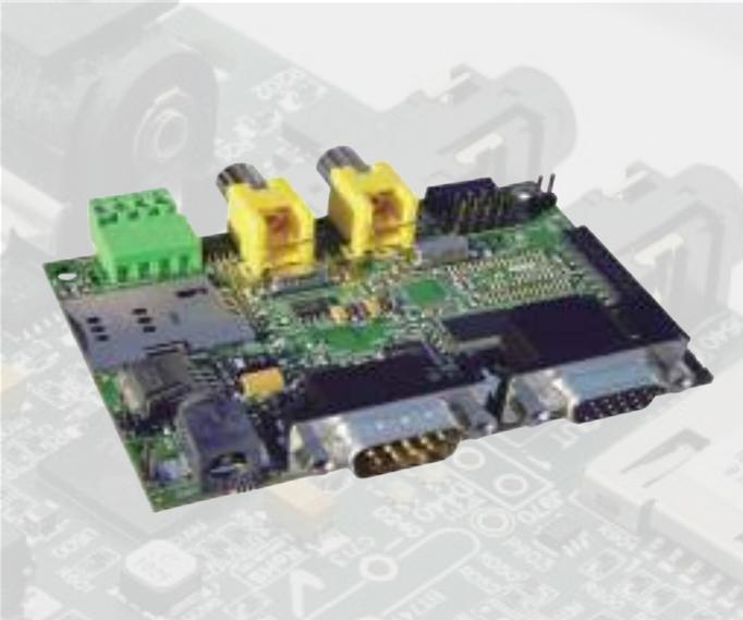
This expansion board has been designed to be used as a test and development complementary platform of IGEP™ v2 DM3730. It can be used to check the final application in pre-prototyping phase, saving costs and reducing time-to-market.
