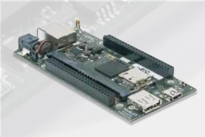
The IGEP™ AQUILA EXPANSION is a fully equipped baseboard that access to all IGEP™ COM AQUILA functionalities. It has been designed to be used as a reliable test and development platform and it can be used as the fastest way to develop and check the user's final application before building a prototype, saving costs and reducing time-to-market.
